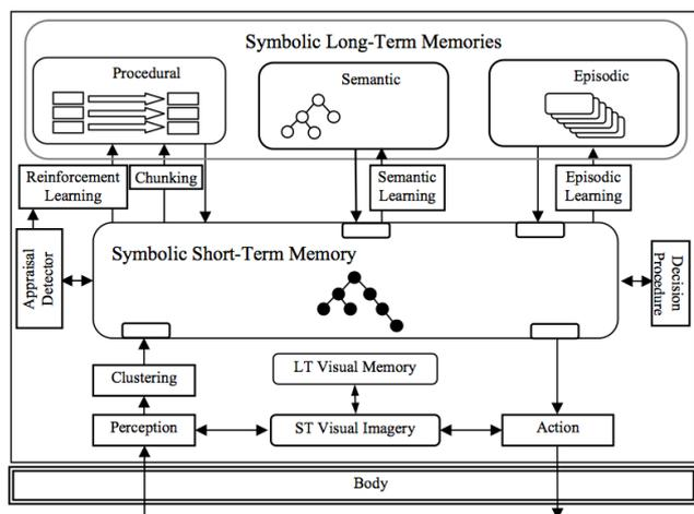
**Figure 1: The structure of the Soar cognitive architecture.**
