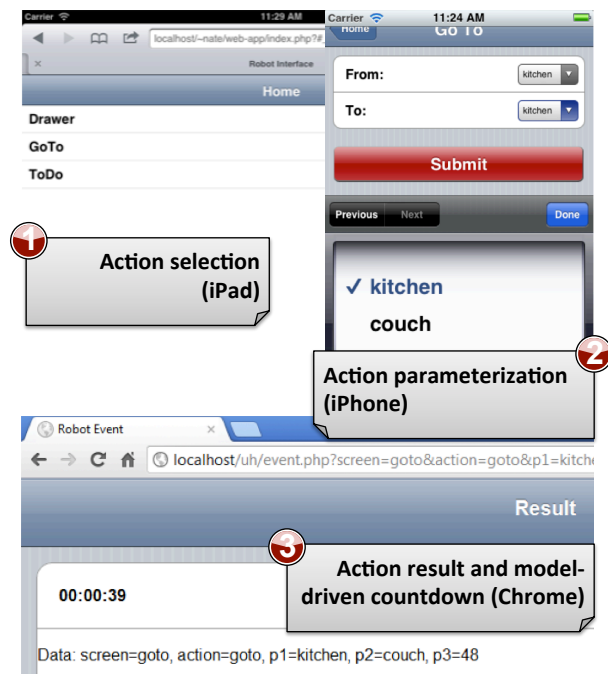
Figure 3. Robot-interaction and virtual-sensor interface (sequence of screenshots for an action on three different devices/programs).
